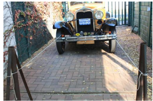
Figure 4: Two strings pulled taut in front of the front wheels.
