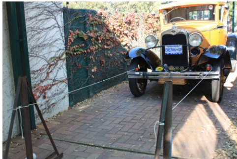
Figure 4: Two strings pulled taut in front of the front wheels.
