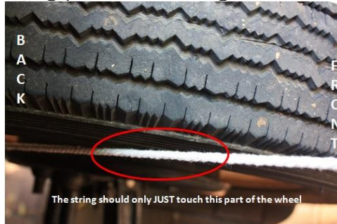
Figure 3: String pulled taut from inside of the wheel to the weighted pole in front of that wheel
