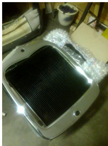
Shiny new radiator surround, re-cored radiator
