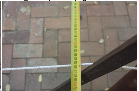
Figure 5: Measure the distance between the strings, close to the car, and then at the measured distance near the weighted poles
