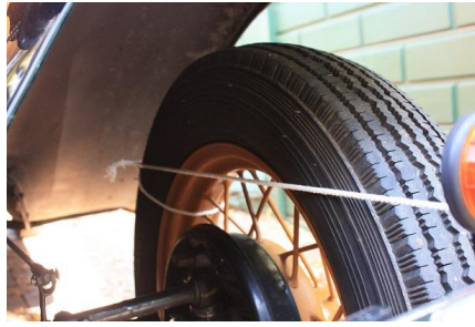
Figure 2: Fasten the string at the top half of the wheel.
