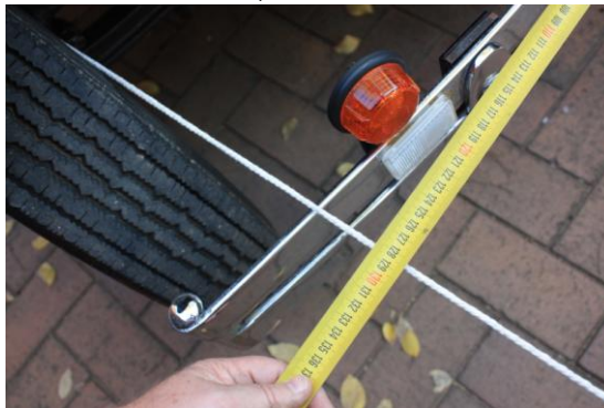
Figure 5: Measure the distance between the strings, close to the car, and then at the measured distance near the weighted poles
