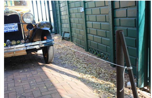
Figure 3: String pulled taut from inside of the wheel to the weighted pole in front of that wheel
