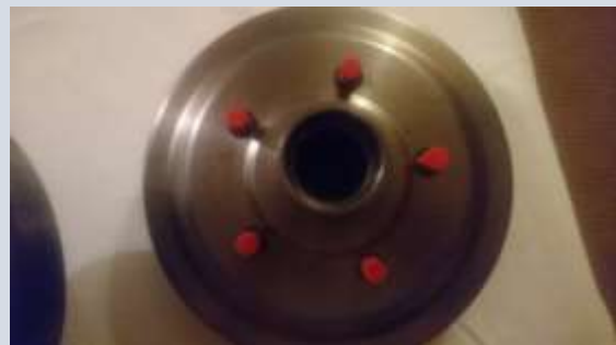
A set of new front hubs and drums, with studs already swaged on
